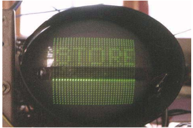
Williams Tube on the replica Manchester Mark I
